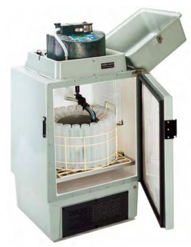
For automatic documentation of sample storage temperature, specify the 6712FR with optional temperature sensor. With this thermally ballasted sensor, the 6712 controller can log compartment temperatures at programmable intervals with 0.1°C precision.
